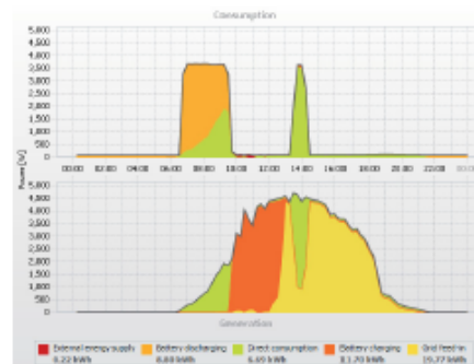
Figure 10 Energy balance in Vlotho (15.06.2015) [12]
